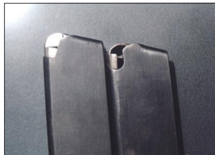
The two types of magazines are illustrated in this photograph. The solid follower type (left) gave better feed results. The incline of the feed path is a bit higher with this follower.
