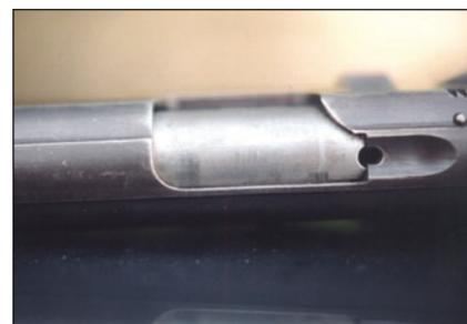
The Star Modelo Super incorporates a loaded chamber indicator in the design. In this illustration the chamber is empty.
